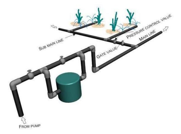
FIGURE 10. The sprinkler irrigation system
