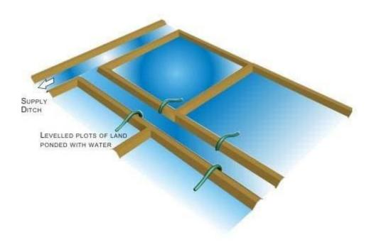
FIGURE 7. Check basin method of irrigation
