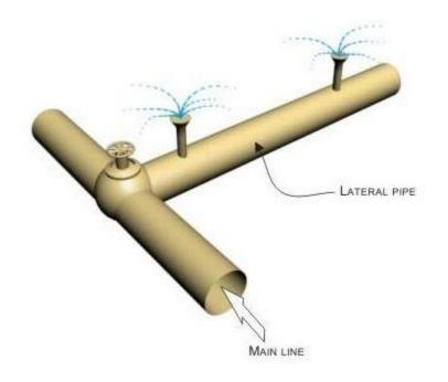
FIGURE 12. Rotating head system of sprinkler irrigation
