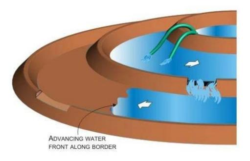
FIGURE 6. Contour border method of irrigation
